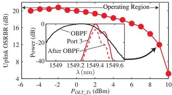
Fig. 7. Influence of backscattering on the uplink channel performance. The inset illustrates that the system's resilience to SBS is a direct result of the offset filter, as its characteristic 10 GHz frequency offset sets it further down the stop band. The OBPF profile is included for reference.
