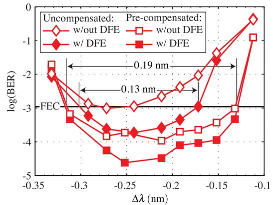
Fig. 5. The impact of offset filtering and spectral pre-compensation on the uplink BER.  $\Delta\lambda = \lambda_{filter} - \lambda_{UL}$ , where  $\lambda_{filter}$  is the filter passband centre and  $\lambda_{UL}$  is the uplink channel's peak wavelength.  $P_{OLT\_Tx} = 5$  dBm.
