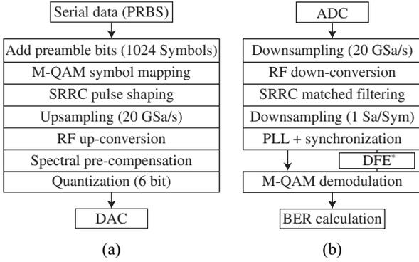
Fig. 2. Block diagrams of the (a) transmitter and (b) receiver DSP stacks used for offline processing of the downlink and uplink signals. \*Note that DFE post-compensation is not performed on the received downlink signal.
