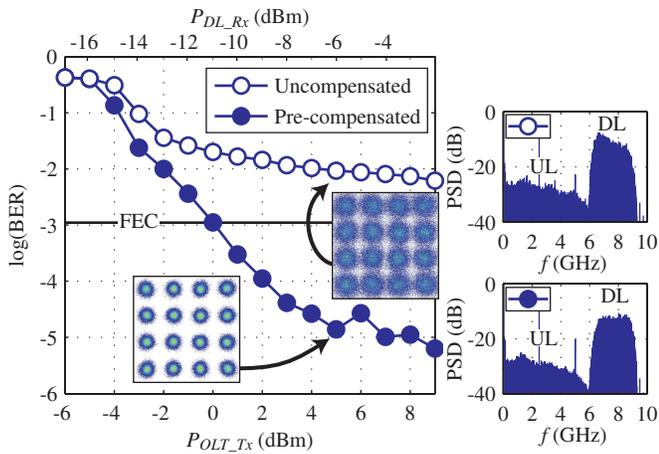
Fig. 3. BER performance of the 2.5 Gbaud 16-QAM downlink transmissions after 20 km. Constellation diagrams and electrical power spectra at  $P_{OLT\_Tx} = 5$  dBm are inset as indicated. The corresponding  $P_{DL\_Rx}$  at the ONU indicates a received power sensitivity of  $-11$  dBm. We note the presence of uplink channel RB noise due to the simultaneous upstream transmission.
