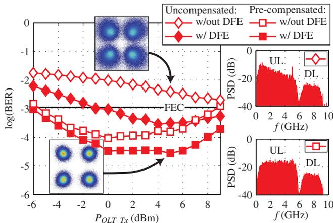
Fig. 4. BER performance of the uplink channel with and without spectral pre-compensation for the RSOA. Constellation diagrams and electrical power spectra at  $P_{OLT\_Tx} = 5$  dBm are inset as indicated. The OBPF is offset by  $-0.18$  nm resulting in an average loss of 6.6 dB, including insertion losses. We also note the presence of the residual downlink channel which was amplified and reflected by the RSOA.
