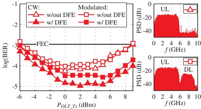
Fig. 6. Comparison of the uplink BER performance with CW and modulated downlink seed light. Electrical power spectra at  $P_{OLT\_Tx} = 5$  dBm are inset as indicated.  $\Delta\lambda = -0.18$  nm.
