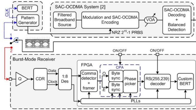
Fig. 1. Block diagram of  $7 \times 622$  Mb/s SAC-OCDMA experimental setup with the BMRx. PLL: phase-locked loop.
