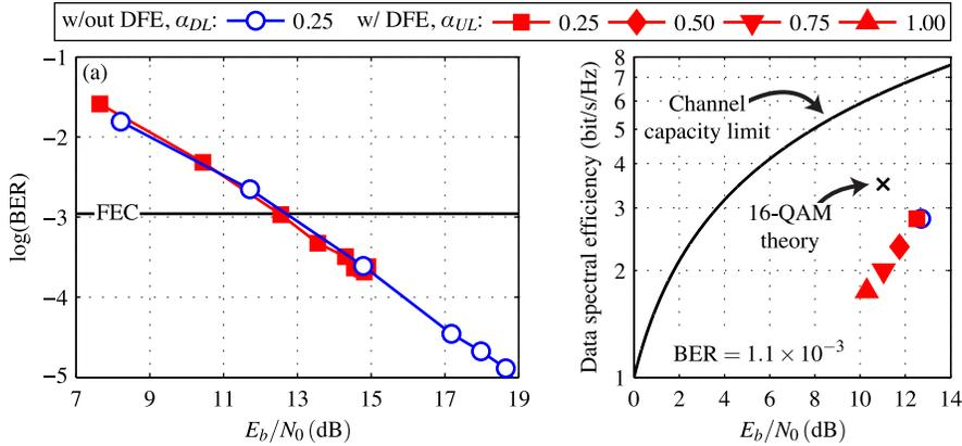
Fig. 5. (a) BER vs.  $E_b/N_0$  for the downlink and uplink channels. (b) Comparison of the 16-QAM SCM WDM PON performance with different SRRC roll off factors to Shannon's channel capacity limit. We also include the best theoretical 16-QAM RS(255,223) FEC coded signal to achieve the BER threshold [23]. Note that the added overhead for the RS(255,223) FEC has been taken into account for both the spectral efficiency and  $E_b/N_0$ .
