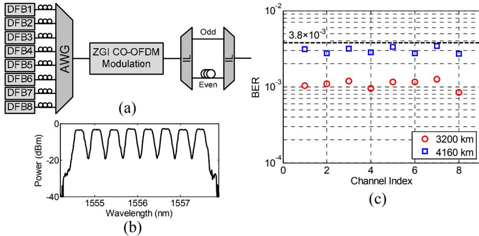
Fig. 6. (a) The transmitter for the WDM transmission. IL: interleaver. (b) The spectrum of the generated 8-channel WDM signal. (c) The BER performance of all channels.
