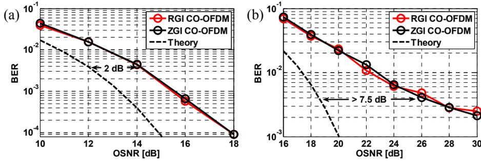
Fig. 3. Measured BER vs. OSNR (0.1nm) for (a) QPSK and (b) 16-QAM signals.
