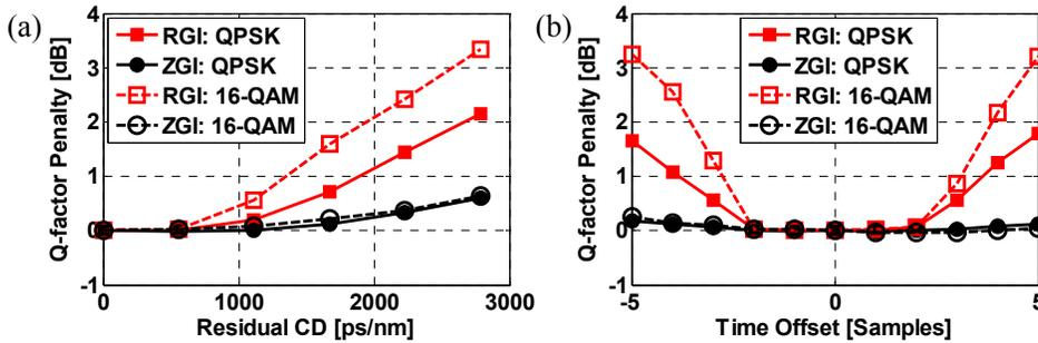
Fig. 5. Measured Q-factor penalty vs. (a) residual CD and (b) time offset. QPSK: 5120 km. 16-QAM: 1280 km.
