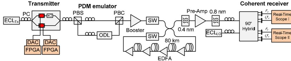
Fig. 2. Experimental setup. ECL: external cavity laser. PC: polarization controller. PBS/PBC: polarization beam splitter/combiner. ODL: optical delay line. SW: switch.
