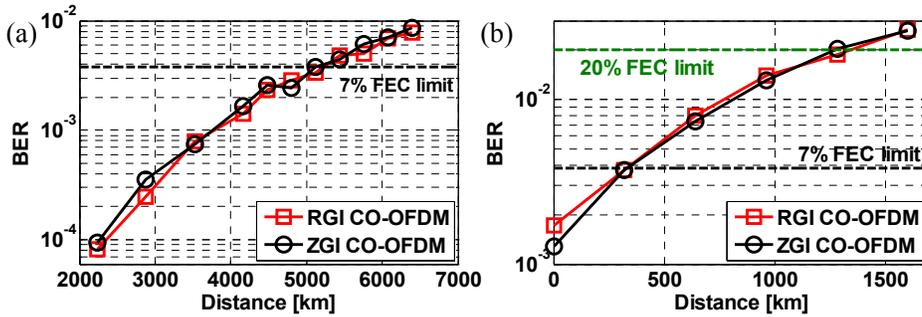
Fig. 4. Measured BER vs. transmission distance for (a) 28 Gbaud QPSK and (b) 16-QAM signals.
