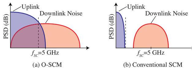
Fig. 4. Illustration of the downlink noise tolerance for (a) this O-SCM WDM PON and (b) a conventional asymmetric SCM PON. The dashed vertical line represents the cutoff frequency for the receiver's electrical low pass filter.
