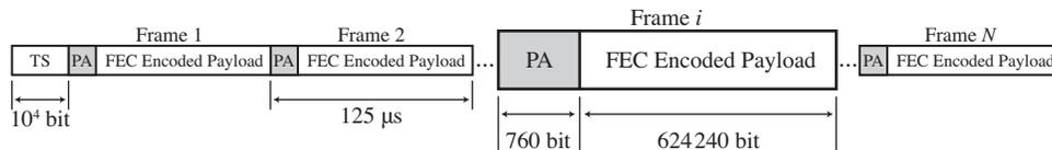
Fig. 2. Illustration of the data structure transmitted at 5 Gb/s. The sequence begins with a  $10^4$  bit training sequence (TS) followed by a series of  $N$  data frames. Each frame is composed of a 760 bit preamble (PA) and a 624 240 bit RS(255,239) FEC encoded payload.
