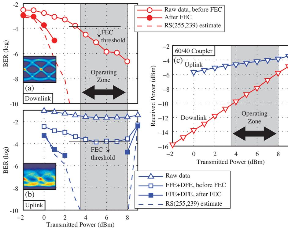
Fig. 3. BER performance as a function of OLT transmitted power in (a) downlink and (b) uplink directions for 5 Gb/s symmetric transmission over 20 km. The inset eye diagrams are of the raw data captured at  $P_{Tx} = 5$  dBm. (c) The corresponding received uplink and downlink power versus transmitted power for the optimum 60/40 coupler.
