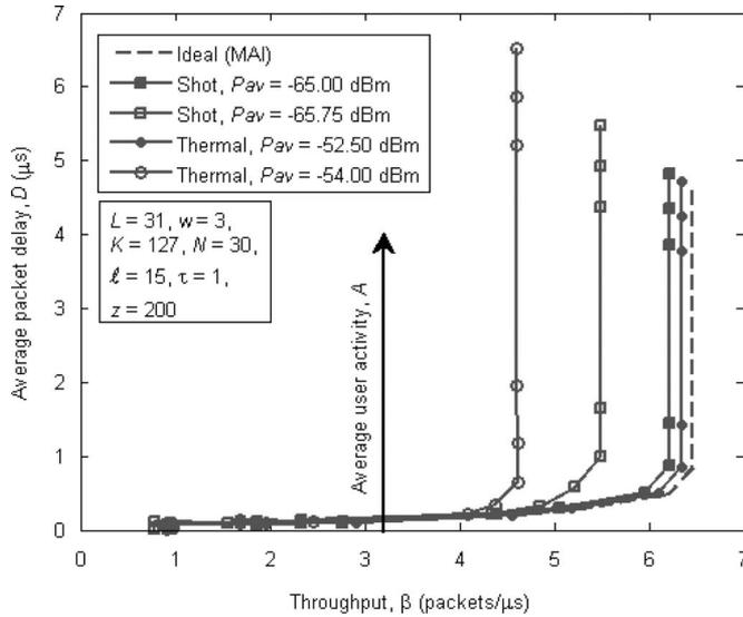
Fig. 4. Packet delay vs. system throughput.
