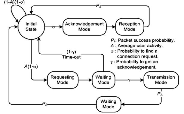
Fig. 1. Simplified state diagram of  $R^3T$  protocol.
