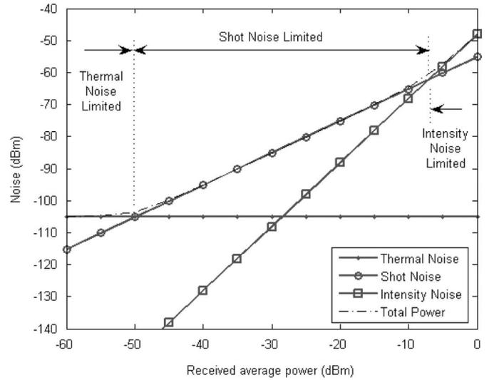
Fig. 6. Noise power vs. received power for different noise sources.
