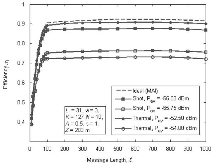
Fig. 5. Efficiency vs. message length for different power levels.
