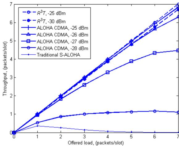
Fig. 2. Throughput versus offered load for different power levels.
