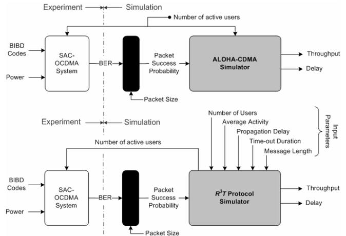
Fig. 1. The experiment/simulation environment.
