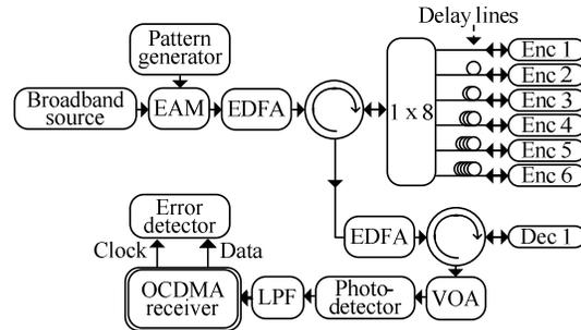
Fig. 1. Experimental setup. EAM: electro-absorption mod., VOA: variable-optical att., LPF: low-pass filter.
