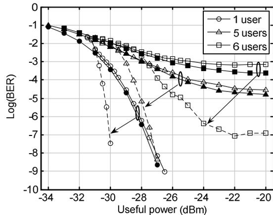
Fig. 4. BER with global clock (solid lines, filled markers), with recovered clock no FEC (solid lines, empty markers) and with recovered clock and FEC (dashed lines, empty markers).
