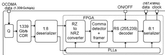
Fig. 3. Block diagram of the OCDMA receiver. The blocks within the dotted area were implemented on an FPGA. Q: quantizer, RS: Reed-Solomon, PLL: phase-locked loop.
