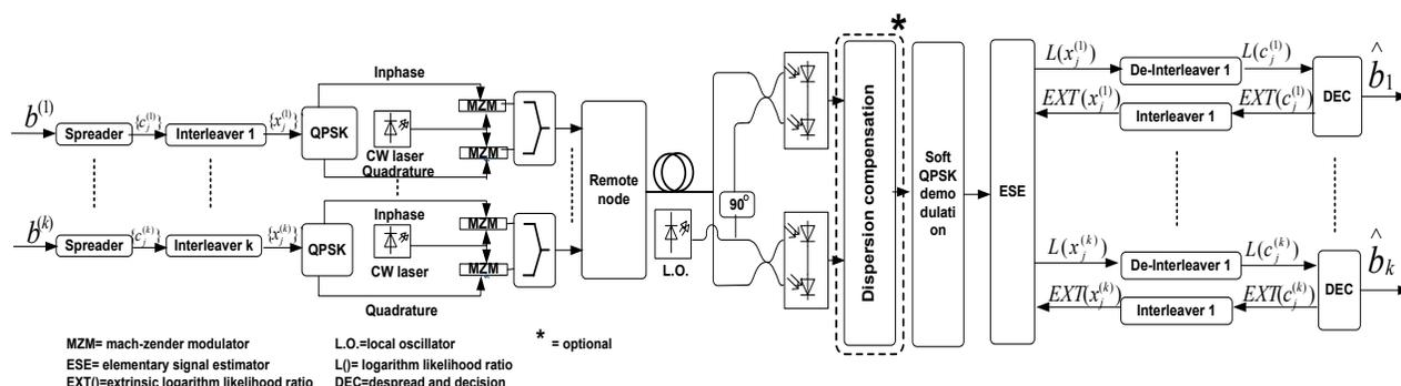
Fig. 1. Architecture of the proposed coherent OIDMA-PON with electronic dispersion compensation (uplink direction).
