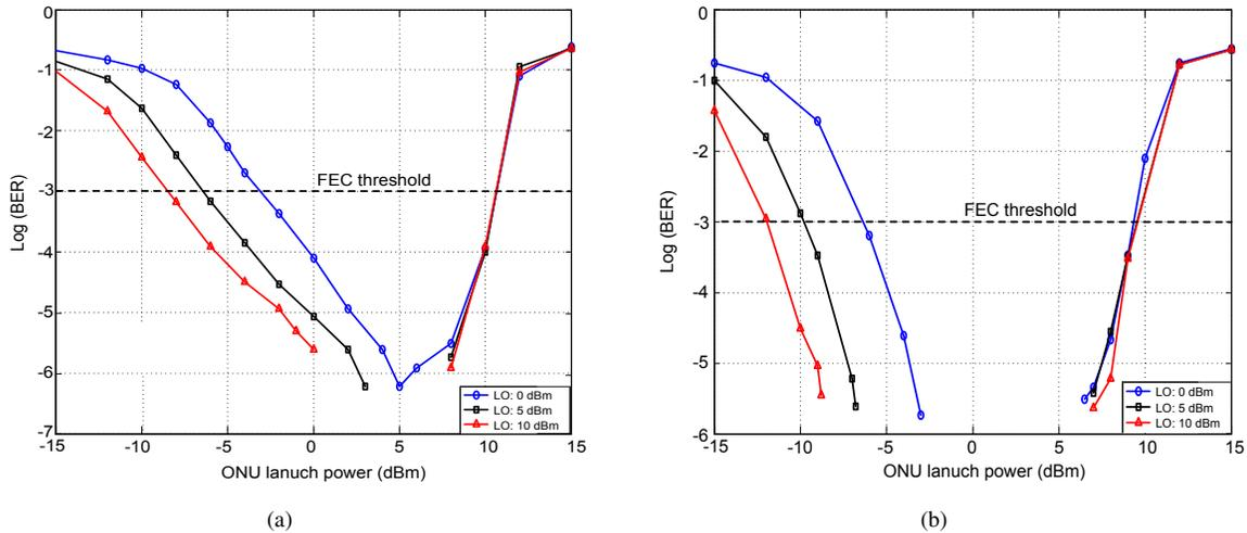
Fig. 3. BER 64 user OIDMA system for 150 km reach versus ONU launch power (a) without dispersion compensation and (b) with electronic dispersion compensation.
