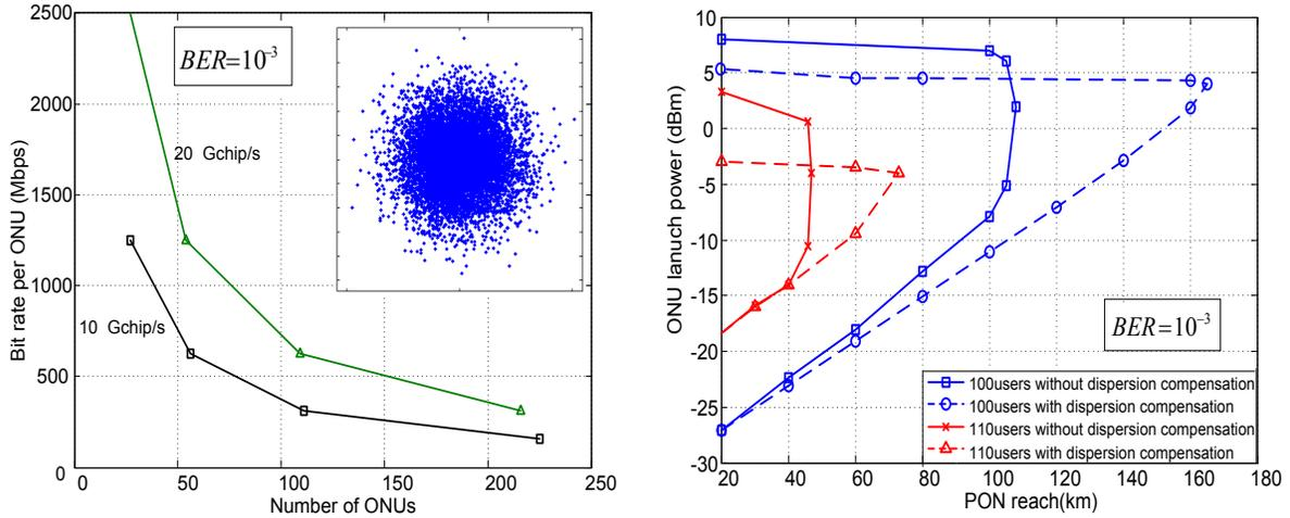
(a) User bit rate versus number of ONUs at 10 and 20 Gchip/s for 100 km reach with electronic dispersion compensation. The inset shows the constellation diagram of the received signal for 100 users at -5 dBm launch power.
