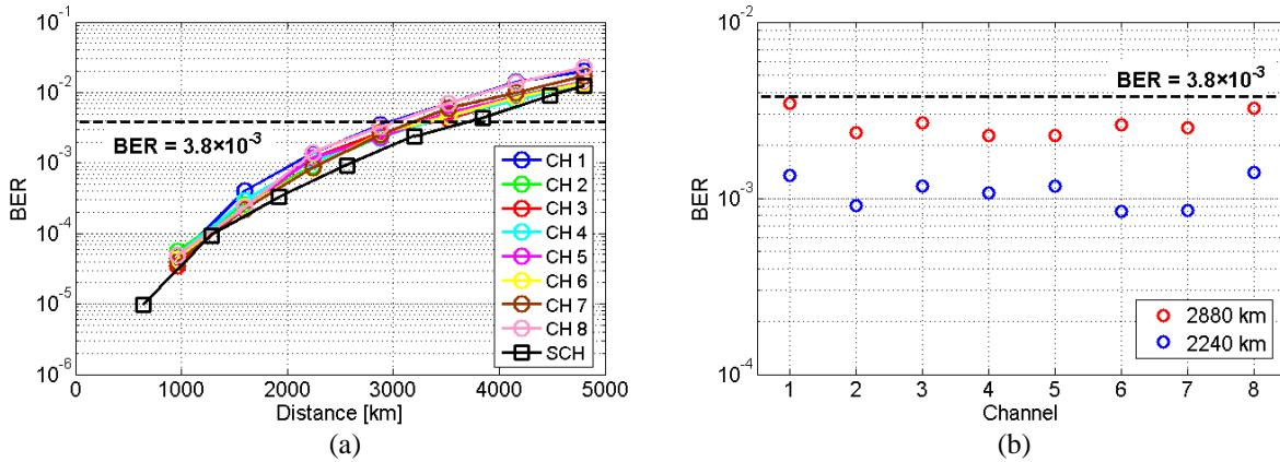
Fig. 3. (a) BER versus distance for the single channel (SCH) transmission and the eight channels in the WDM transmission. (b) The BERs of all channels after 2880 km and 2240 km WDM transmissions.
