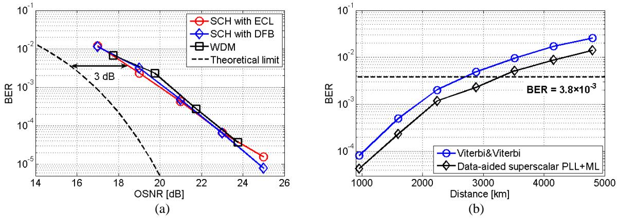
Fig. 2. (a) BER versus OSNR in back-to-back transmission. SCH: single channel. (b) Comparison of the transmission performance with different phase recovery.
