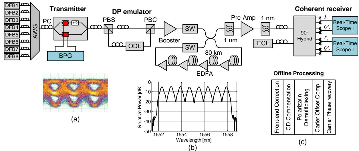
Fig. 1. Experimental setup. ODL: optical delay line, PBS/PBC: polarization beam splitter/combiner, PC: polarization controller, SW: switch. Insets: (a) single-polarization optical QPSK eye diagram; (b) optical spectrum of the eight WDM channels; (c) the offline processing procedures.
