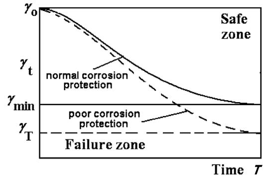
Figure 7. Deterioration of  $\gamma$ .
