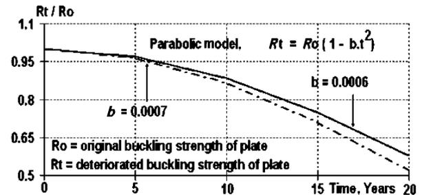
Figure 8. Deterioration of buckling strength.
