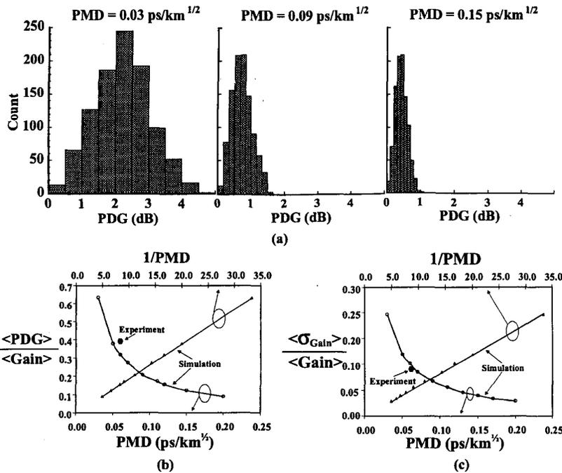
CTuJ1 Fig. 3. (a) Histograms showing how the mean and standard deviation of the Raman PDG decrease as the PMD is increased from 0.03 to 0.09 to 0.15 ps/km<sup>1/2</sup>; (b) and (c) show the mean PDG and the standard deviation of the Raman gain versus PMD (and 1/PMD) for a 10-km Raman amplifier (where the PDG and gain are normalized to the average gain).
