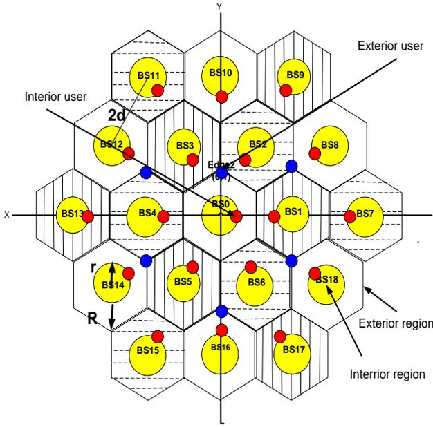
Fig. 2. Two-tier network with FFR three
