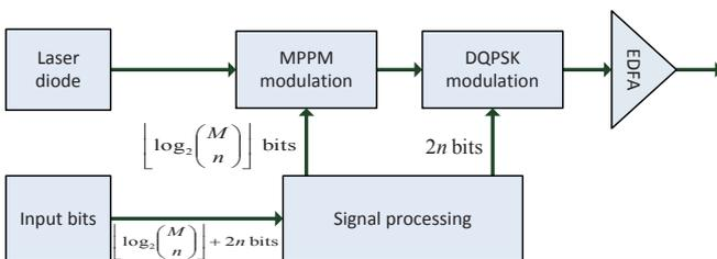
Fig. 1: Block diagram of the hybrid DQPSK-MPPM transmitter.
