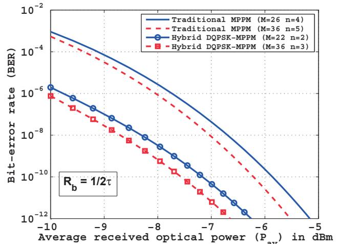
Fig. 5: Average bit-error rate versus average received optical power for both hybrid DQPSK-MPPM and traditional MPPM systems with  $\sigma_n^2 = 1.6 \times 10^{-5} A^2$ .
