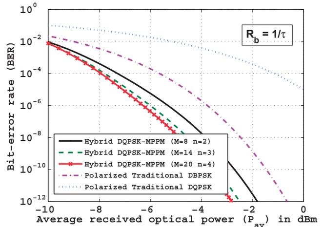
Fig. 4: Average bit-error rate versus average received optical power for proposed DQPSK-MPPM systems, traditional DBPSK, and traditional DQPSK systems with  $\sigma_n^2 = 1.6 \times 10^{-5} A^2$ .
