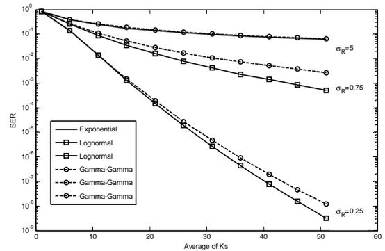
Fig. 2. Average SER versus average of  $K_S$  using the approximate method for different channel models.
