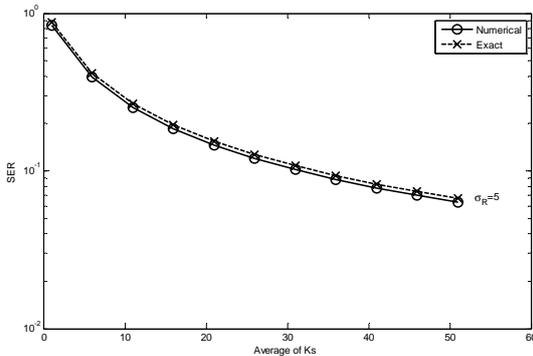
Fig. 1. Average SER versus average of  $K_S$  using exact and approximated method under gamma-gamma distribution with  $M = 8$ ,  $n = 4$ , and  $K_b = 1$ .
