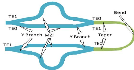
Fig. 1: Schematic diagram of proposed low-order mode suppressor.
