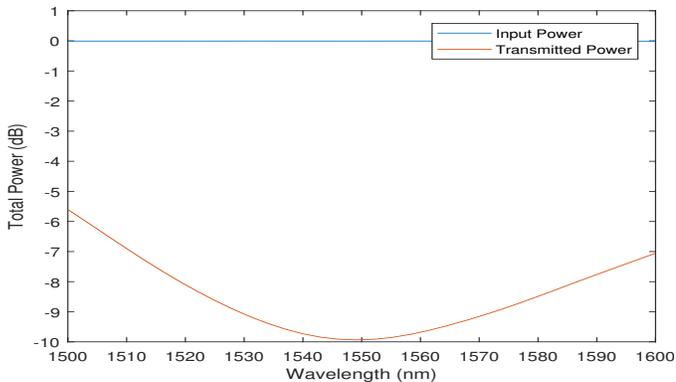
Fig. 2: Transmitted power (dB) versus wavelength (nm) when inserting  $TE_0$  mode.
