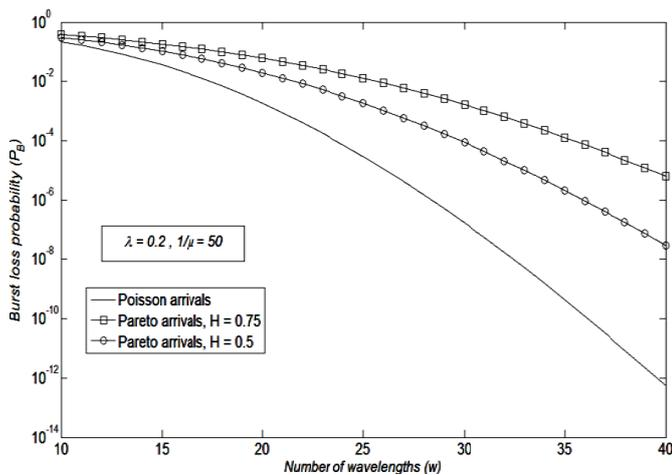
Fig. 3. Burst loss probability versus the number of wavelengths for FWC case for Poisson and Pareto arrivals at different values for the Hurst parameter.
