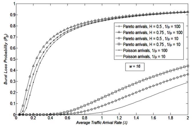
Fig. 2. Burst loss probability versus the average traffic arrival rate for FWC case for Poisson and Pareto arrivals at different values for the Hurst parameter and burst length.
