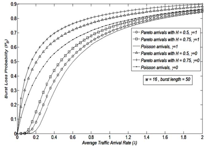
Fig. 1. Burst loss probability versus the average traffic arrival rate for NWC and FWC cases for Poisson and Pareto arrivals at different values for the Hurst parameter.
