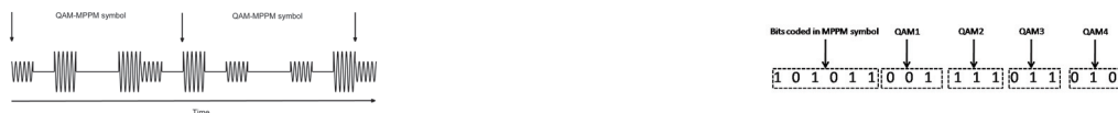
(a) Frame structure of a hybrid QAM-MPPM modulation scheme (b) An example for hybrid QAM-MPPM with (N, w, M_q) = (8, 4, 8) .
