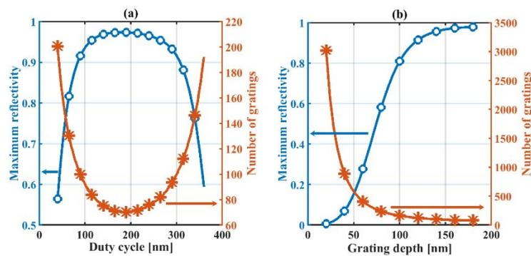
Figure 3. Variation of maximum reflectivity and number of gratings versus: (a) duty cycle; (b) grating depth.
