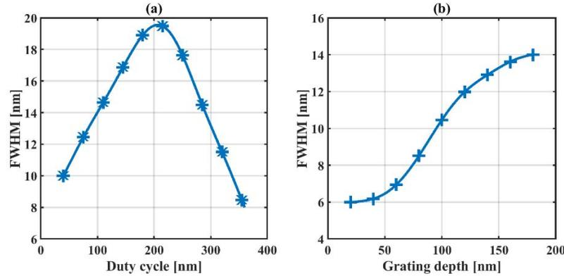
Figure 4. Variation of the FWHM versus: (a) duty cycle; (b) grating depth.
