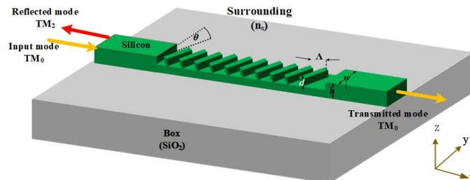
Figure 1. Schematic structure of tilted Bragg grating engrooved into strip silicon waveguide.
