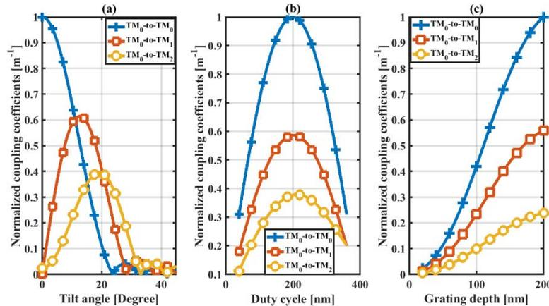
Figure 2. Variation of coupling coefficients versus: (a) tilt angle; (b) duty cycle; (c) grating depth.
