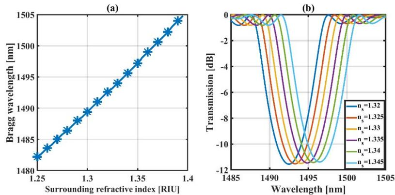
Figure 5: (a) Variation of the Bragg resonance with surrounding refractive index; (b) Spectral response of tilted Bragg grating for different surrounding refractive indices.
