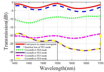
Fig. 2: Insertion loss for TE<sub>1</sub> mode conversion
