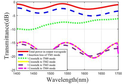
Fig. 3: Insertion loss for TM<sub>1</sub> mode conversion
