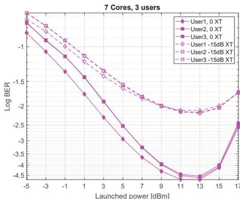
Fig. 4: BER versus launched power  $P_{Tx}$  for 3 users in 7 cores in MCF at 0 and  $-15$  dB crosstalk level.
