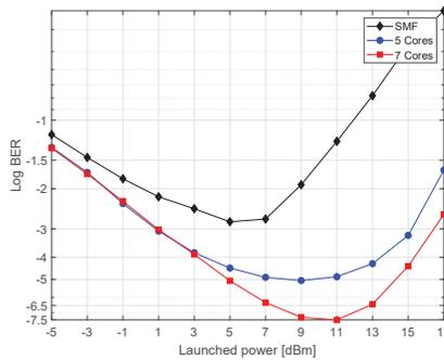
Fig. 2: BER versus launched power  $P_{Tx}$  for 5 and 7 cores in MCF.
