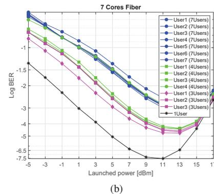
Fig. 3: (a) BER versus launched power  $P_{Tx}$  for 1, 2, 3, and 5 users in 5 cores in MCF. (b) BER versus launched power  $P_{Tx}$  for 1, 3, 4, and 7 users in 7 cores in MCF.
