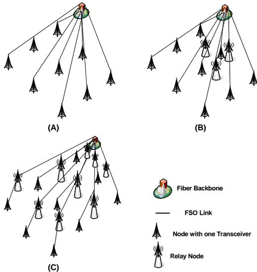
Figure 2: Different recent static topologies at last-mile, (A) Direct Link model (D-L), (B) Partial Relayed Link Model (P-L), (C) Full Relayed Link Model (F-L).
