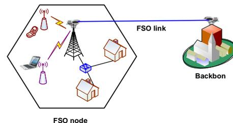
Figure 1: Last-mile FSO connection, the end users could use wire or wireless connections to FSO node.
