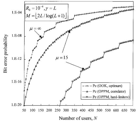
Fig. 7. A comparison between the bit error probabilities of the OPPM-CDMA correlator receivers (with and without optical hardlimiters) and the OOK-CDMA optimum receivers versus the number of simultaneous user when  $\gamma = L$  and  $M = \lfloor 2L / \log(L + 1) \rfloor$ .
