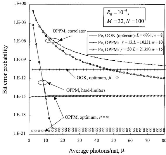
Fig. 4. A comparison between the bit error probabilities of the OPPM-CDMA correlator receivers (with and without optical hardlimiters) and both the OOK- and OPPM-CDMA optimum receivers versus the average photons per nat.
