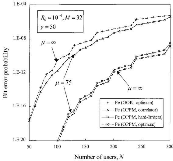
Fig. 5. A comparison between the bit error probabilities of the OPPM-CDMA correlator receivers (with and without optical hardlimiters) and both the OOK- and OPPM-CDMA optimum receivers versus the number of simultaneous user.
