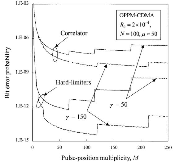
Fig. 6. A comparison between the bit error probabilities of the OPPM-CDMA correlator receivers (with and without optical hardlimiters) for two different values of the overlapping index versus the pulse-position multiplicity.
