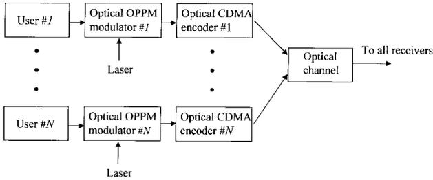
Fig. 1. Optical overlapping PPM-CDMA transmitter model.
