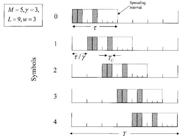
Fig. 2. An example of the transmitted signal formats of single user in an OPPM-CDMA system with  $M = 5$ ,  $\gamma = 3$ ,  $L = 9$ , and  $w = 3$ . A signature code of 110010000 is assumed.
