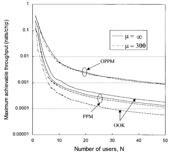
Fig. 8. A comparison between the maximum achievable throughput of optical OOK-, PPM-, and OPPM-CDMA receivers versus the number of users when  $\mu \in \{300, \infty\}$  and the BER does not exceed  $10^{-9}$ .
