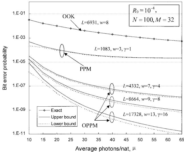
Fig. 6. A comparison between the bit error rates of optical OOK-, PPM-, and OPPM-CDMA receivers (with  $M = 32$  and different values of  $\gamma$  for OPPM) under the constraints of fixed throughput, chip time, and number of users.
