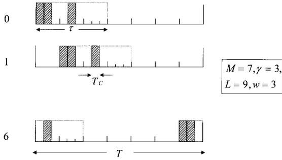
Fig. 5. An example of the transmitted signal formats of a single user in an OPPM-CDMA system with  $M = 7$ ,  $\gamma = 3$ ,  $L = 9$ , and  $w = 3$ . A signature code of 110010000 is assumed.
