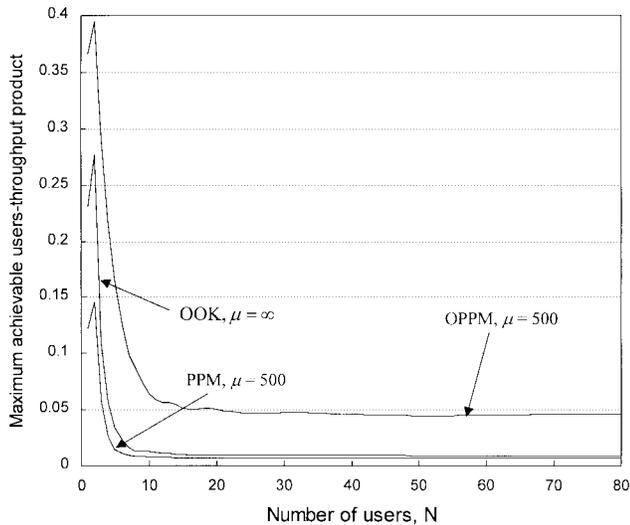
Fig. 9. A comparison between the maximum achievable users-throughput products of optical OOK-, PPM-, and OPPM-CDMA receivers versus the number of users when  $\mu \in \{500, \infty\}$  and the BER does not exceed  $10^{-9}$ .
