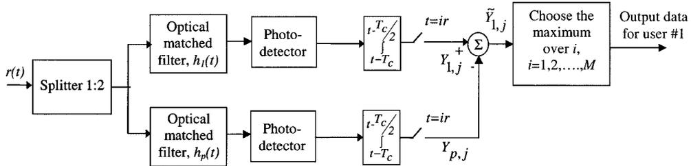
**Figure 2** Direct-detection optical PPM-CDMA system model with interference cancellation
