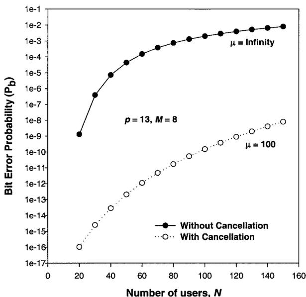
**Figure 4** PPM-CDMA BER variations versus the number of simultaneous users for  $p = 13$  and  $M = 8$ . For the system without cancellation [1], a lower bound is evaluated at  $\mu = \infty$ . For the system with cancellation, an upper bound is evaluated at  $\mu = 100$
