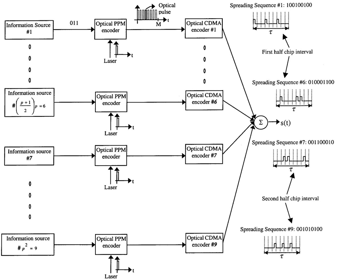
**Figure 1** Optical PPM-CDMA transmitter system with alternate Manchester coding (8-ary PPM CDMA, with prime code sequence length of 9 ( $p = 3$ ); information source #1 sending symbol 4 (011 bits), and the prime code sequence of source #1 is 100010001)
