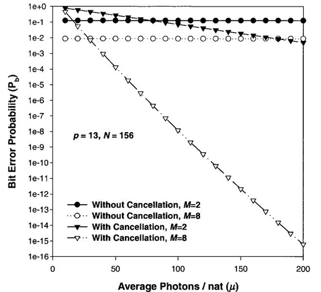
**Figure 3** Comparison between lower bounds on the BER of PPM-CDMA systems without cancellation [1] and upper bounds on the BER of PPM-CDMA systems with cancellation (with and without Manchester codes) for  $p = 13$  and  $N = 156$  (full load condition). The lower bounds are evaluated at  $\mu = \infty$
