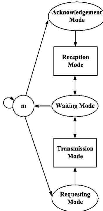
Fig. 3. Block diagram of the  $R^3T$  protocol.
