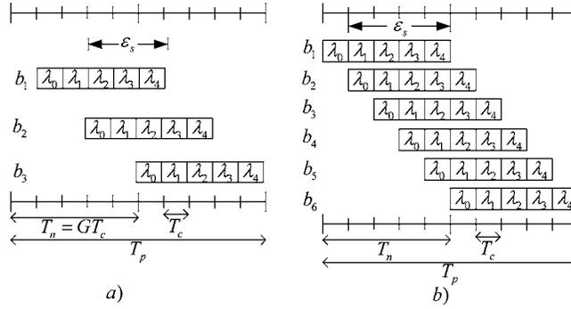
Fig. 5. Optical overlapped OFFH-CDMA packet model of a single user in a given time slot: (a)  $\varepsilon_s=3$ , (b)  $\varepsilon_s=4$ .
