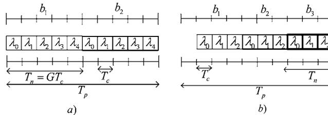
Fig. 4. Optical VPG-OFFH-CDMA packet model of a single user in a given packet time slot: (a)  $G_V=5$ , (b)  $G_V=3$ .
