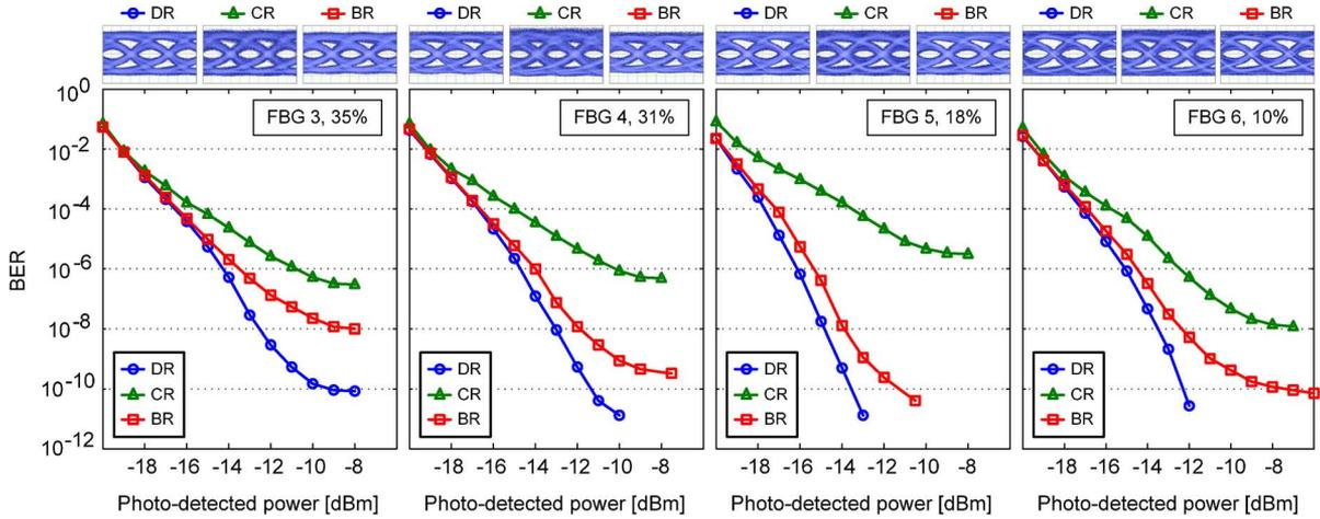
Fig. 6. Back-to-back BER performance corresponding to the same FBGs in Fig. 5 when using the three receiver options (BR: balanced receiver, CR: conventional receiver, DR: degenerate receiver).
