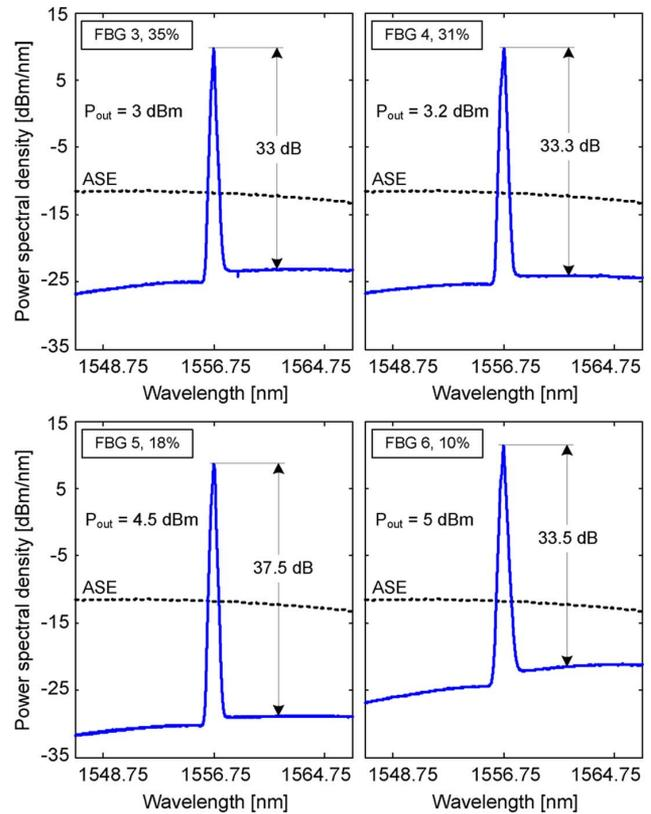
Fig. 5. Power spectral density at the output of our proposed self-seeded RSOA transmitter for FBGs with 35%, 31%, 18%, and 10% reflectivities, compared to the output ASE from the RSOA without self-seeding.
