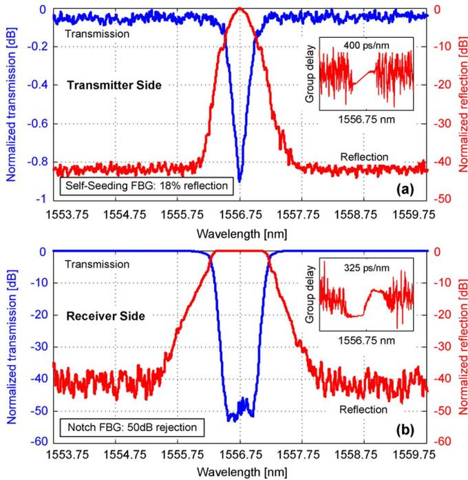
Fig. 4. Characterization of the 18% self-seeding FBG used at the transmitter and the FBG used with both the BR and the CR.
