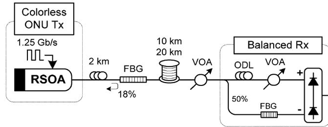
Fig. 9. Experimental setup for remote self-seeding.
