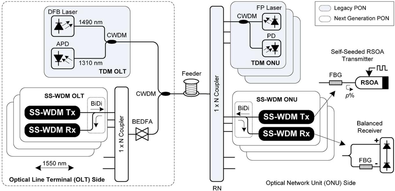
Fig. 3. Hybrid dense SS-WDM PON and TDM PON over the existing PON infrastructure (APD: avalanche photodiode, BEDFA: bidirectional EDFA, BiDi: bidirectional, CWDM: coarse WDM, DFB: distributed feed-back, FBG: fiber Bragg grating, FP: Fabry-Perot, PD: photodiode, Rx: receiver, Tx: transmitter).
