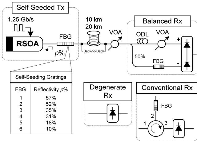
Fig. 2. Experimental setup showing our self-seeded RSOA transmitter with the three receiver structures under test and a table with the FBGs used for self-seeding (ODL: optical delay line, VOA: variable optical attenuator).
