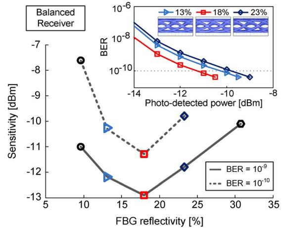
Fig. 7. Sensitivity versus FBG reflectivity for the BR.
