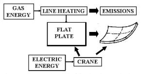
Figure 11 Energy demand of line heating method
