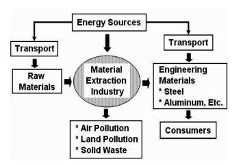
Figure 2. Energy & environment of pre-production stage
