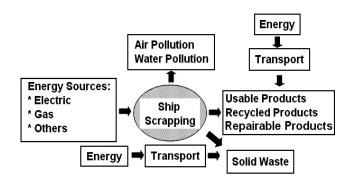
Figure 20. Energy and environment in ship demolition stage
