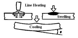
Figure 12. Principle of line heating method
