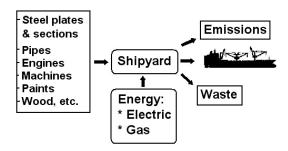
Figure 6. Input /output of a shipyard
