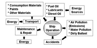
Figure 16. Energy and Environment in ship operation
