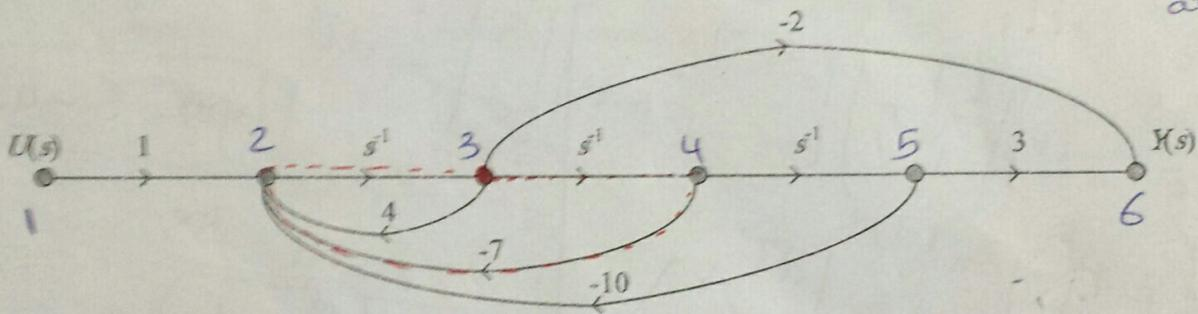
③ a. Find the transfer function  $\frac{Y(s)}{U(s)}$  using Mason's gain formula.
