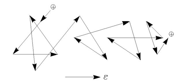
• *Drift* is the motion caused by an electric field.
