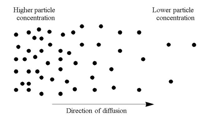
Particles diffuse from a higher-concentration location to a lower-concentration location  $\rightarrow$  <u>There must be</u> <u>concentration gradient for diffusion to occur (e.g. Non-</u> <u>uniform doping)</u>
