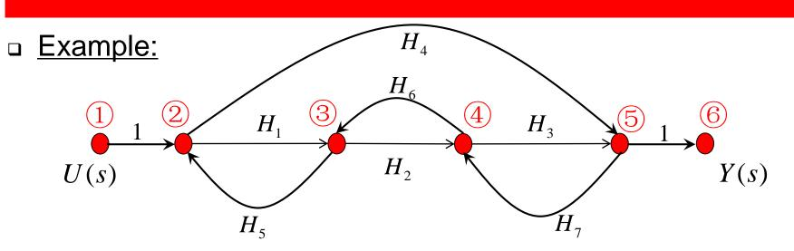
Forward path Path gain  $G_1 = H_1 H_2 H_3$  $G_2 = H_4$ Loop path Path gain  $l_1 = H_1 H_5$  $l_2 = H_2 H_6$  $l_3 = H_3 H_7$  $l_4 = H_4 H_7 H_6 H_5$
