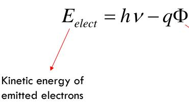
Workfunction of metal (minimum energy required to release an electron from the barrier)
