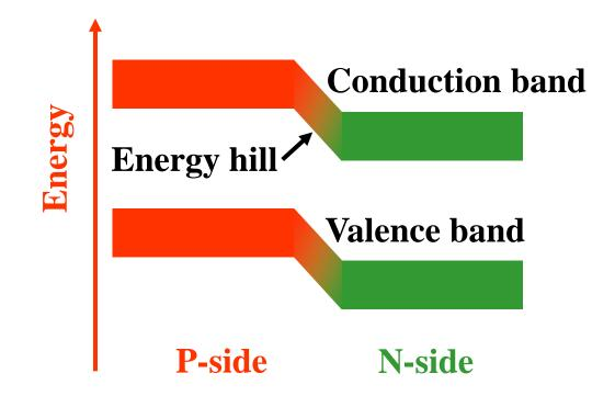
To an electron trying to diffuse across the junction, the path it must travel looks like an energy hill. It <u>must</u> receive the extra energy from an <u>outside</u> source.
