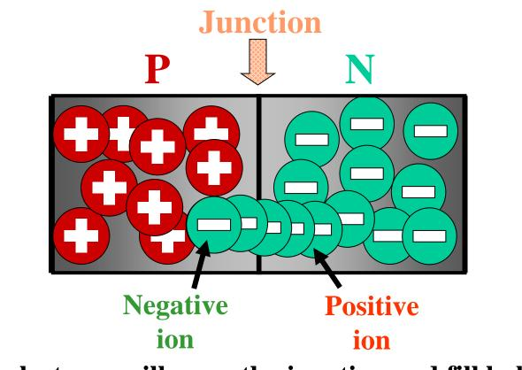
Some electrons will cross the junction and fill holes. A pair of ions is created each time this happens. As this ion charge builds up, it prevents further charge migration across the junction.
