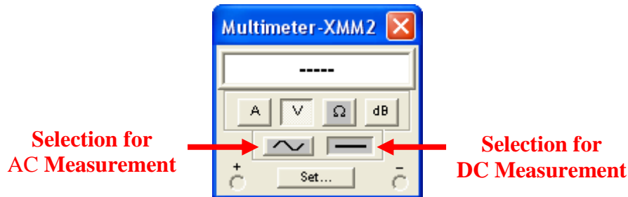
Figure 15: Multimeter properties window
