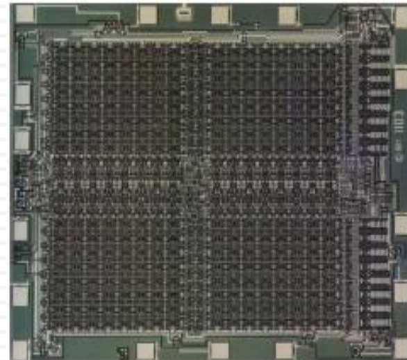
Figure 0.5 Intel 1103 1K-bit DRAM
