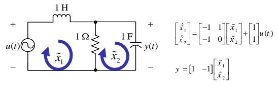
State variables are:  $\tilde{x}_1:$  current of left loop,  $\tilde{x}_2:$  current of left loop
