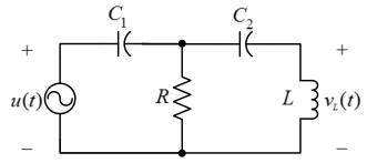
Input variables (Input voltage u(t)), Output variables (Inductor voltage  $v_L(t)$ )
