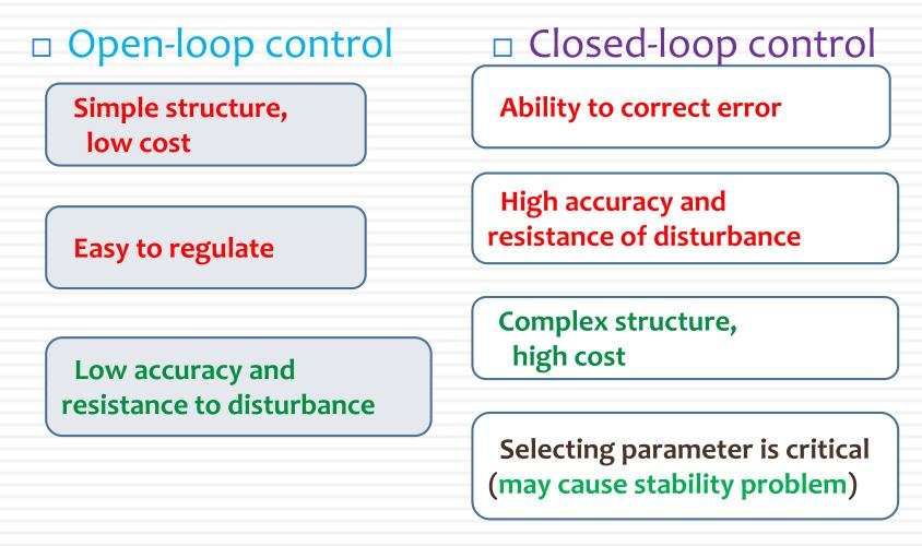
Open-loop + Closed-loop = Composite control system
