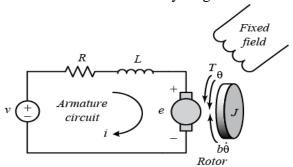
We will assume that the input of the system is the voltage source (V) applied to the motor's armature, while the output is the rotational speed of the shaft d(theta)/dt.
