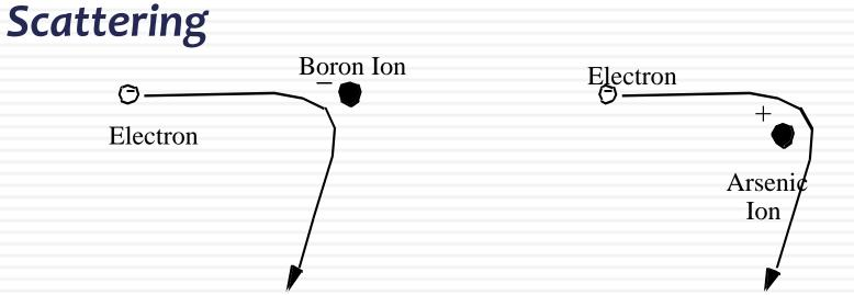
There is less change in the direction of travel if the electron zips by the ion at a higher speed.
