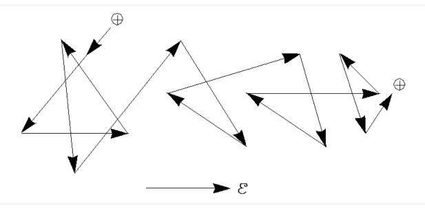
• *Drift* is the motion caused by an electric field.
