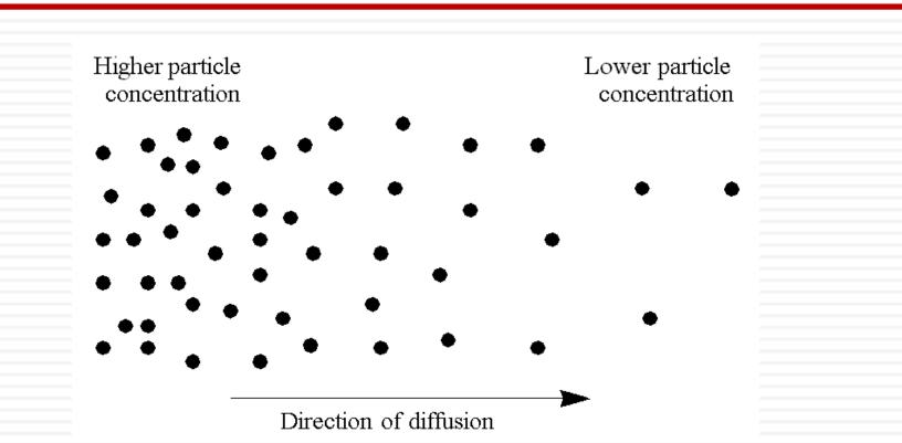
Particles diffuse from a higher-concentration location to a lower-concentration location.
