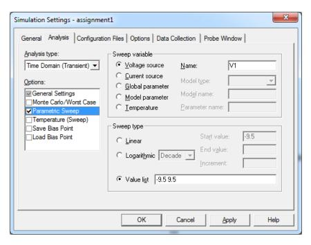
16.Run a DC sweep on the voltage source from -9.5V to 9.5V, comment on the results.
