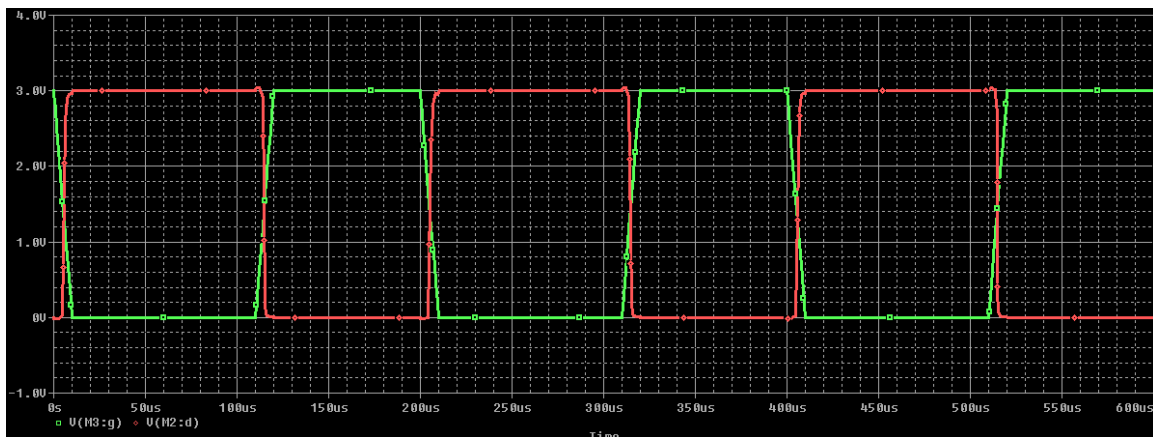
Figure 2 CMOS inverter input and output waveforms
