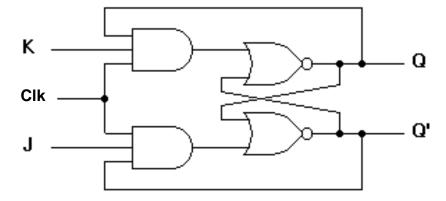
b) Establish the truth table of the JK latch of part (a) indicating each mode of operation.
