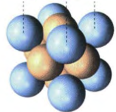
Face-centred Cubic Unit Cell (FCC)
