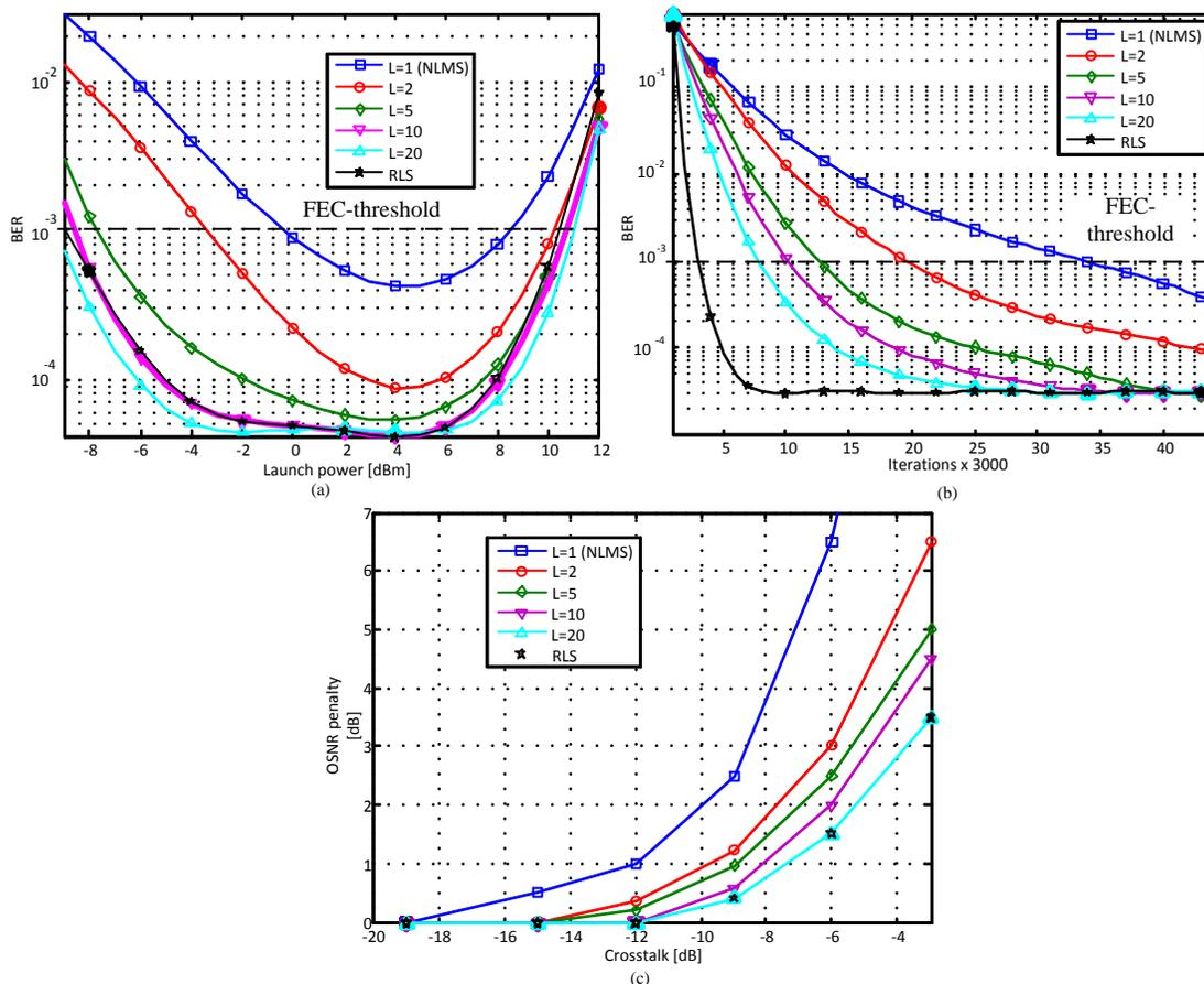
Fig. 2 (a) BER vs. Launch power in dBm for NLMS, APA with  $\mu=0.001$  and RLS with forgetting factor  $\lambda=0.999$  at  $XT=-6.5$  dB, (b) BER vs. number of iterations, and (c) OSNR penalty vs. crosstalk at 0.1 nm resolution bandwidth; launch power is taken at the min BER.
