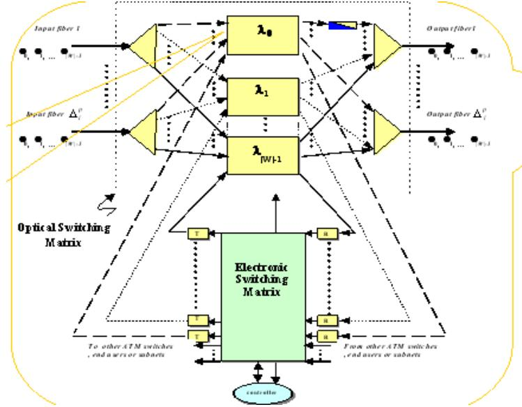
Figure 1. Wavelength Convertible Optical Switch.
