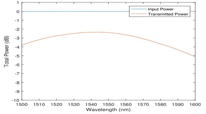
Fig. 3: Transmitted over (dB) versus wavelength (nm) when inserting a  $TE_0$  mode.
