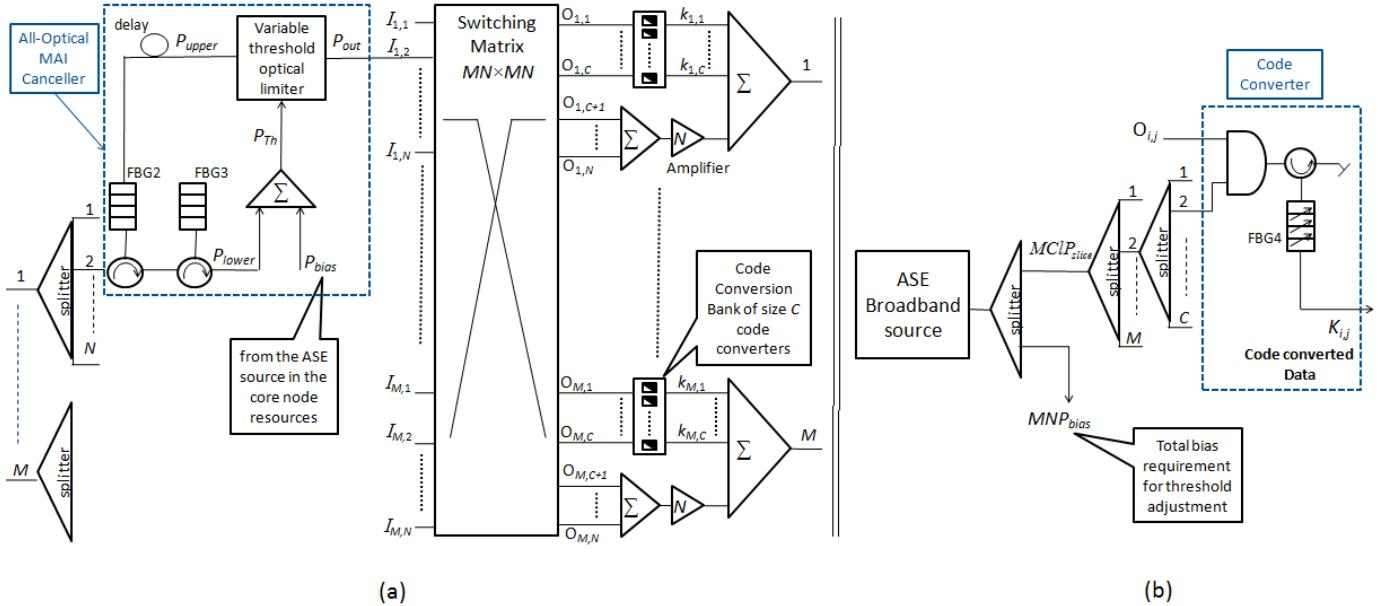
Fig. 3. Architecture of a core node in OBS/SAC-OCDMA system.
