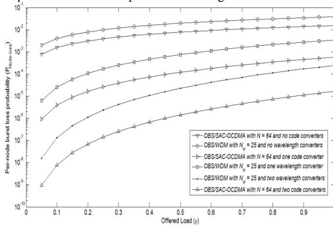
Fig. 5. Semi-log plot for MAC layer *per-node burst loss probability* versus the Offered Load for OBS/SAC-OCDMA and OBS/WDM systems at different number of code and wavelength converters.
