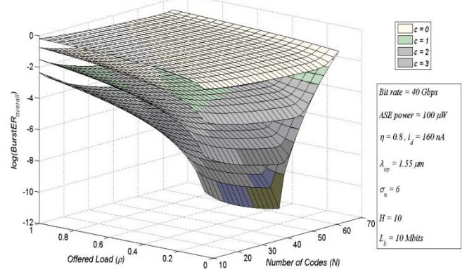
Fig. 7. Log *overall burst error rate* versus both the available number of codes and the offered load for OBS/SAC-OCDMA system at different number of code converters.
