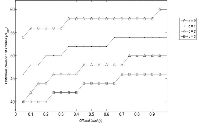
Fig. 8. Optimum number of codes versus the offered load at different number of code converters employed.
