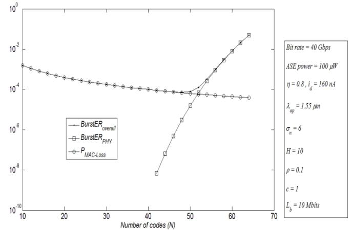
Fig. 6. Semi-log plot of *MAC burst loss probability*, optical layer *burst error rate* and *overall burst error rate* versus the available number of codes for OBS/SAC-OCDMA system with one code converter.
