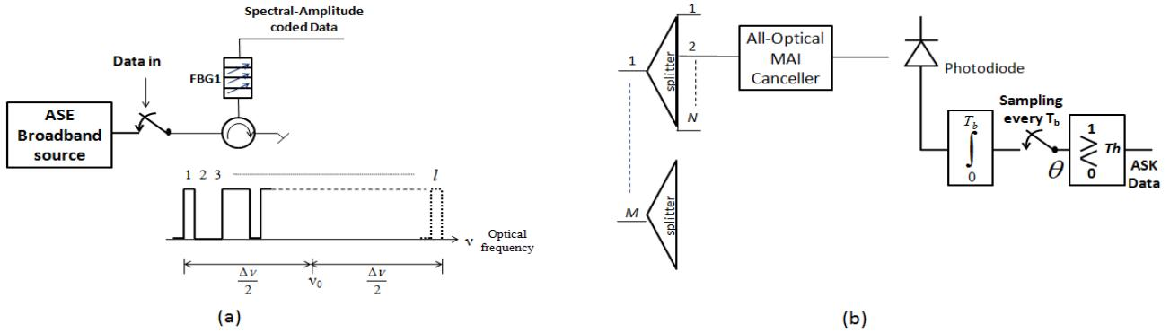
Fig. 2. Architecture of an edge (ingress/egress) node in OBS/SAC-OCDMA system.
