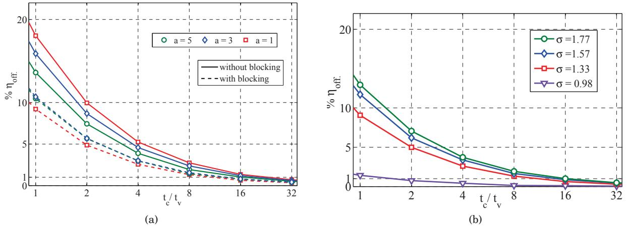
Fig. 2. Offloading efficiency for cellular/LiFi HetNet versus the ratio  $t_c/t_v$  at: (a) different values of variability parameter ( $a = 1, 3$ , and,  $5$ ) with and without LiFi blocking consideration; (b) different level of users' density of  $\sigma = 1.77, 1.33, 1.57$ , and  $0.98$ , at a variability parameter of  $a = 1$ , taking LiFi signal blocking into consideration.
