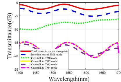
Fig. 3: Insertion loss for  $\text{TM}_1$  mode conversion
