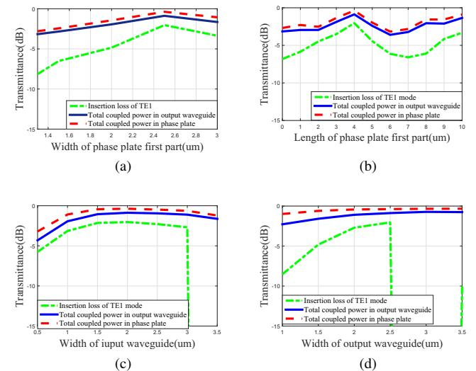
Fig. 4: FDTD simulation sweep for design parameters: (a) sweep for width of first part of phase plate, (b) sweep for length of first part phase plate, (c) sweep for width of input waveguide, and (d) sweep for width of output waveguide.
