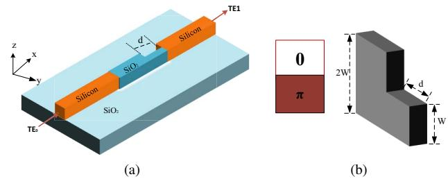
Fig. 1: (a) Schematic diagram of proposed structure, (b) Phase pattern of first-order mode with cross-sectional area of phase plate.
