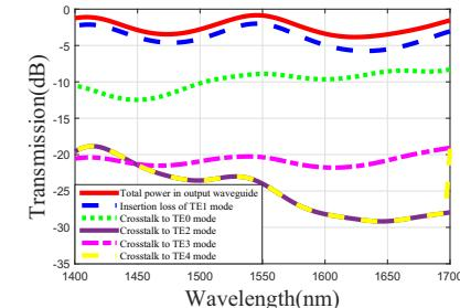
Fig. 2: Insertion loss for  $\text{TE}_1$  mode conversion
