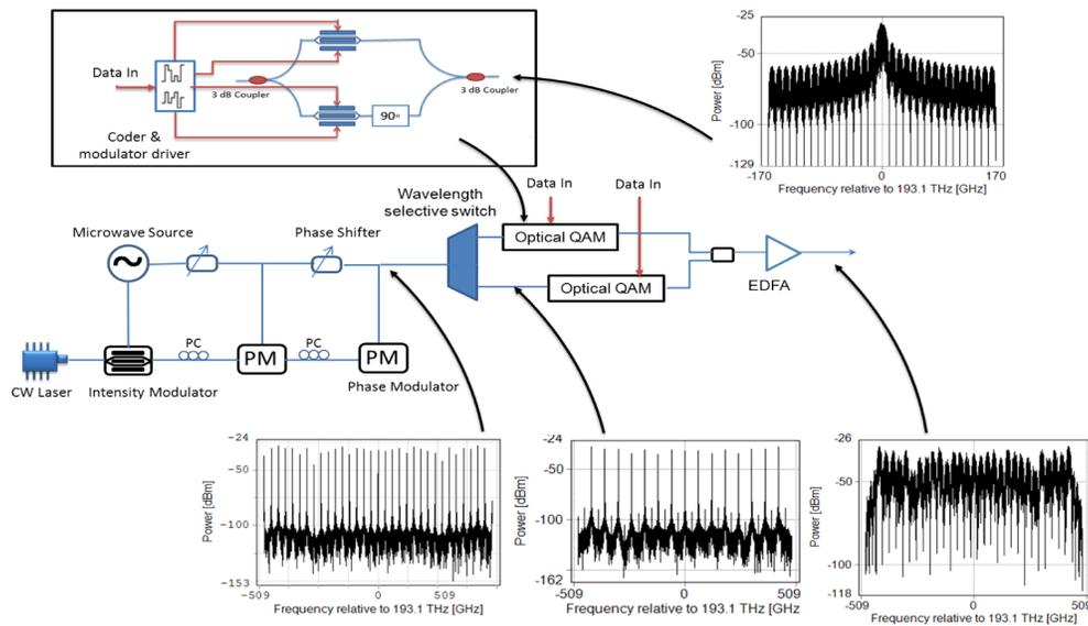
Fig. 1. Transmitter of an all-optical OFDM transmission system.
